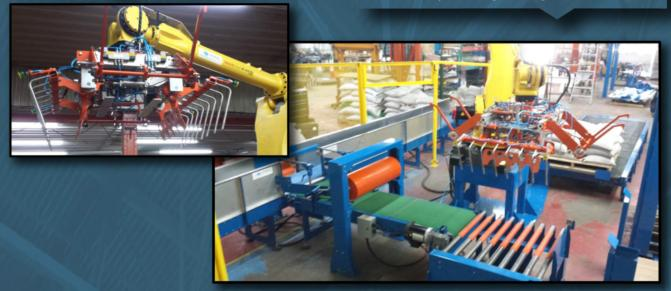
The work of manually palletizing 50 lb. and 100 lb. bags was previously done by 4 operators over 2 shiftsdifficult jobs in a tight labor market. Increased production demands called for a better solution. Solutech gathered the data, custom-designed a robotic palletizing solution, laid out the floor plan out at the customer's facility and provided a real time simulation. Showing the simulation before actually making the project for the customer provided an increased comfort level.
